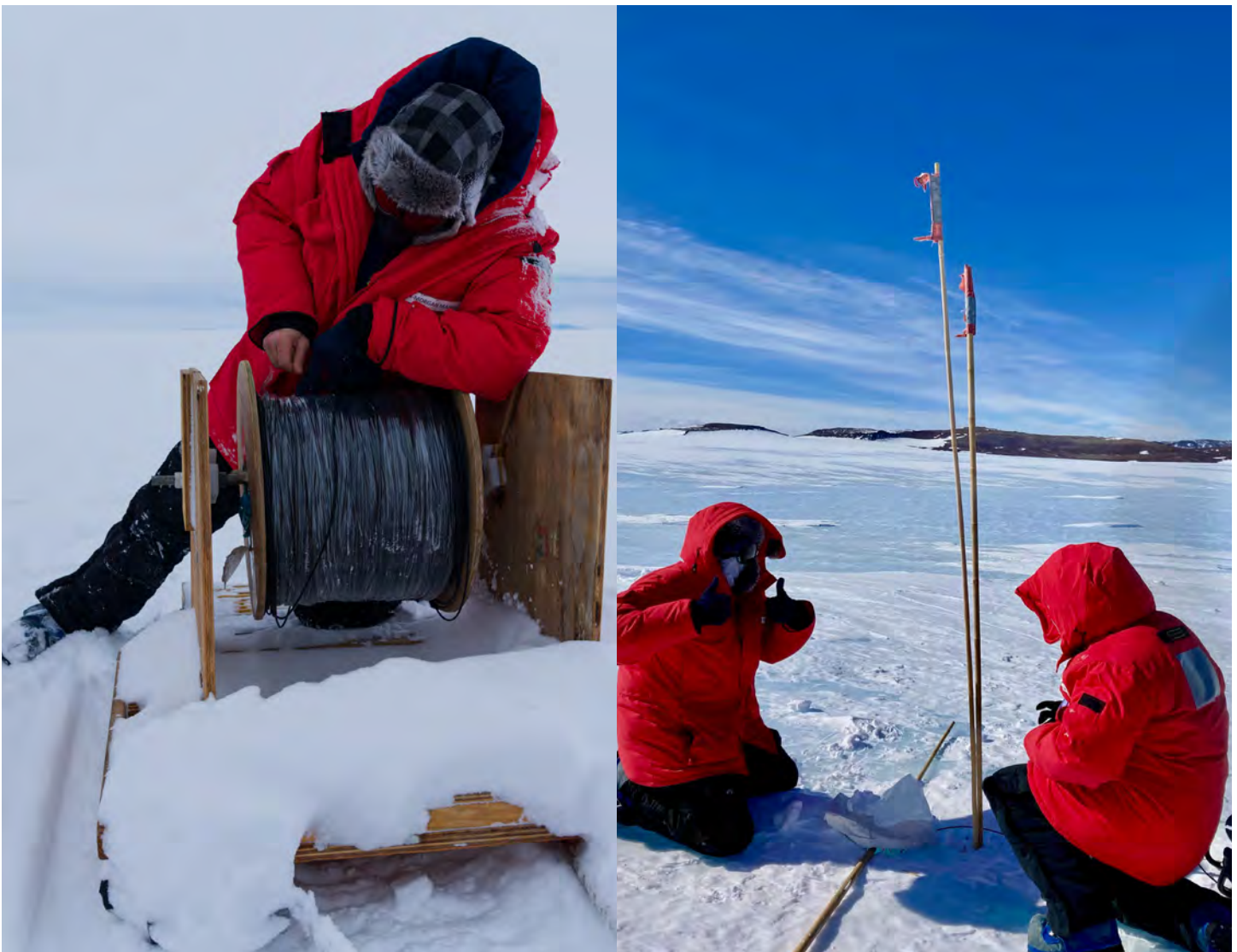
Graduate student John-Morgan Manos on the McMurdo Ice Shelf. The projects in Antarctica included two experiments using fiber optics: 1) a 5 km single mode cable and distributed acoustic sensing (DAS) interrogator were deployed on the McMurdo Ice Shelf and 2) a multimode cable and distributed temperature sensing (DTS) cable were deployed into a previously drilled borehole in the Allan Hills blue ice zone. on McMurdo Ice Shelf, researchers are interested in learning more about the cryoseismic activity of the ice shelf as tidal forces were driving motion. At Allan Hills, they were interested in collecting a high spatial and temporal resolution temperature profile of the ice in this region. Photo credit: John-Morgan Manos
